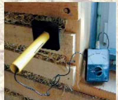
Measuring Moisture in Straw Bale Walls
